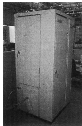
Fig. 7. Package of hot-water supply system.
